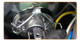
Attach the connector of the low and high beam bulb.
