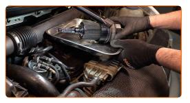
Replacement: engine oil and filter – MERCEDES-BENZ Sprinter Dumptruck (W905). Tip:
