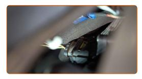
Fasten the clamp on the air intake hose. Use a drive socket #7. Use a ratchet wrench.
