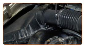
Disconnect the air intake pipe from the air filter housing. Use a crowbar.
