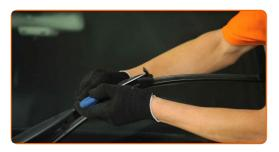
Remove the blade from the wiper arm.
