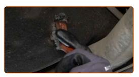
Unscrew the drain plug. Use a drive socket #13. Use a ratchet wrench.
