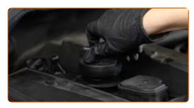
Tighten the oil filler cap.
