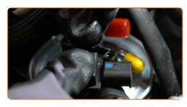
Screw in the water-in-fuel sensor fasteners. Use Torx T20.
