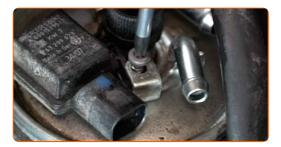
Disconnect the water-in-fuel sensor from the fuel filter.
