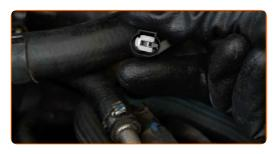
Detach the vacuum valve from its mounting seat and set it aside. Use a crowbar.
