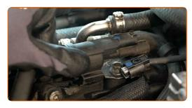
Plug in the vacuum valve connector.
