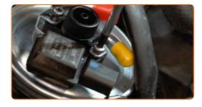
18 Attach the tubes to the fuel filter.
