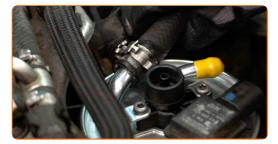
Tighten the fastening clamps of the fuel filter pipes. Use clic-R collar pliers.
