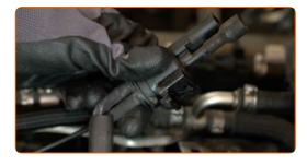
Detach the connector of the water-in-fuel sensor.
