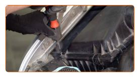
Release the air filter cover clips.
