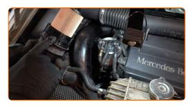
Screw the new filter into its place.
