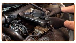
Replacement: engine oil and filter – MERCEDES-BENZ Sprinter 5-T Platform/Chassis (W905). Tip:
