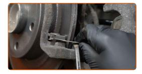
17 Install the retaining springs of the brake pads.
