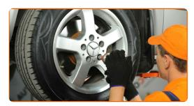
Replacement: brake pads – MERCEDES-BENZ SPRINTER 5-t Platform/Chassis (906). Tip:
