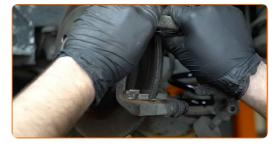
Remove the brake pad wear sensor from the brake pad. Use a flat screwdriver.
