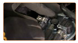
Screw the fastener attaching the fuel supply line to the fuel filter housing. Use a Phillips screwdriver.
