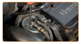
Disconnect the pipe from the fuel filter.
