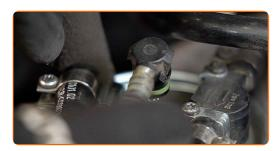
Unscrew the fastener attaching the fuel supply line to the fuel filter housing. Use a Phillips screwdriver.
