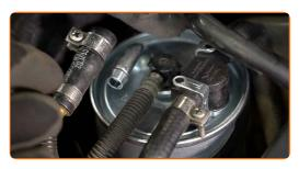
14 Attach the pipe to the fuel filter.
