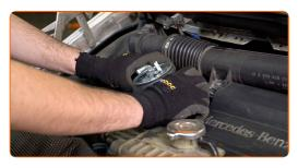
Replacement: fuel filter – MERCEDES-BENZ SPRINTER 5-t Platform/Chassis (905). Tip from AUTODOC experts:
