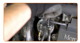
Tighten the fastening clamp of the fuel filter pipe. Use a Phillips screwdriver.
