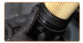
Install the cover of the oil filter housing and screw it on.
