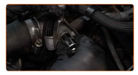
Screw in the bracket fastener. Use Torx E11. Use a ratchet wrench.
