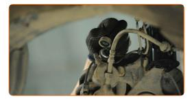
Disconnect the brake pad wear sensor plug. Use round-nose pliers.
