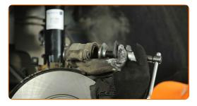
24 Install the brake caliper and fix it.
