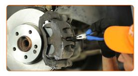
Install the dust boot caps of the brake caliper guide pins. Use a flat screwdriver.
