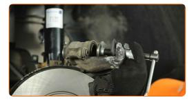
24 Install the brake caliper and fix it.
