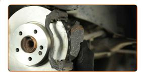
Replacement: brake pads – MERCEDES-BENZ SPRINTER 5-t Box (906).
