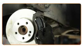
Replacement: brake pads – MERCEDES-BENZ SPRINTER 5-t Box (906).
