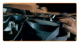
Replacement: serpentine belt – MERCEDES-BENZ Sprinter 4-T Platform/Chassis (W904). Tip from AUTODOC:
