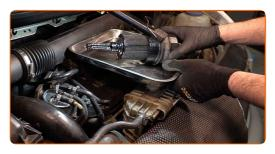
Replacement: engine oil and filter – MERCEDES-BENZ Sprinter 4-T Minibus (W904). Tip:
