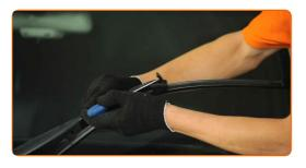
Remove the blade from the wiper arm.
