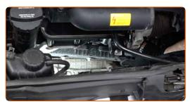
Unscrew the ignition coil bracket. Use a drive socket #E11. Use a ratchet wrench.
