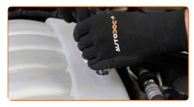
Remove the back section of the engine cover.
