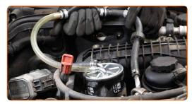
Attach the pipe to the fuel filter.
