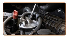
Detach the tubes from the fuel filter. Use round-nose pliers.
