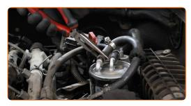
Replacement: fuel filter – MERCEDES-BENZ SPRINTER 3-t Platform/Chassis (906). Tip:
