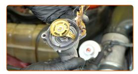
Clean the thermostat housing mounting seat. Use a wire brush. Use all-purpose cleaning spray.
