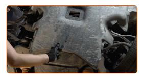
8 Detach the oxygen sensor connector.
