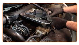
Replacement: engine oil and filter – MERCEDES-BENZ Sprinter 3-T Minibus (W906). Tip:
