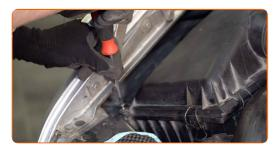
Release the air filter cover clips.
