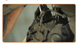
Connect the brake pad wear sensor plug.
