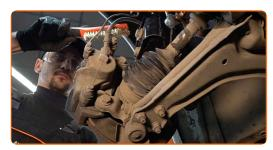
Unscrew the brake caliper fastening. Use HEX No.H6. Use a ratchet wrench.
