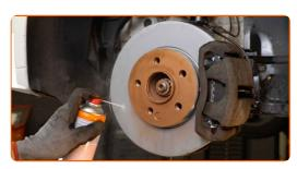
Replacement: brake pads – MERCEDES-BENZ SPRINTER 3-t Bus (907). Tip from AUTODOC experts:
