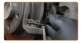
17 Install the retaining springs of the brake pads.
