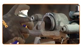
Replacement: brake pads – MERCEDES-BENZ SPRINTER 3-t Bus (907). Tip from AUTODOC:
