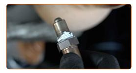
14 Install the new oxygen sensor.
