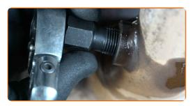
Treat the oxygen sensor. Use high-temperature ceramic grease.
