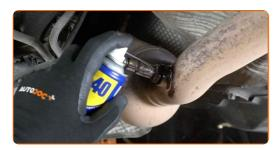
Unscrew the oxygen sensor fastener. Use a 22-mm oxygen sensor socket. Use a ratchet wrench.
