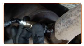
Tighten the oxygen sensor fastener. Use a combination spanner #22. Use a torque wrench. Tighten it to 51 Nm torque.
