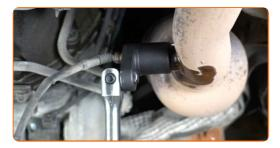
11 Remove the oxygen sensor.
