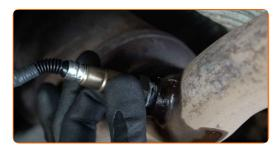
Tighten the oxygen sensor fastener. Use a combination spanner #22. Use a torque wrench. Tighten it to 51 Nm torque.
