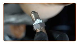
14 Install the new oxygen sensor.
