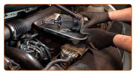
Replacement: engine oil and filter – MERCEDES-BENZ Sprinter 2-T Van (W901, W902). Tip:
