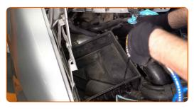
Replacement: air filter – MERCEDES-BENZ Sprinter 2-T Minibus (W901, W902). Professionals recommend:
