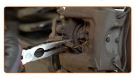
Clean the fasteners of the brake pad wear sensor wiring harness. Use a wire brush. Use WD-40 spray.
