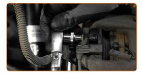
10 Remove the fastening bolt.
