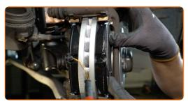
Treat the brake caliper piston. Use a nylon cleaning brush. Use a brake cleaner.
