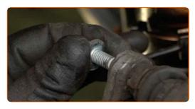
Tighten the brake caliper fasteners. Use a combination spanner #17. Use a drive socket #13. Use a torque wrench. Tighten it to 34 Nm torque.
