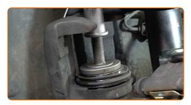
Install the brake caliper and fix it. Use a drive socket #12. Use a torque wrench. Tighten it to 25 Nm torque.
