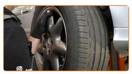
Detach the connector of the brake pad wear sensor. Use round-nose pliers.
