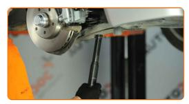
Tighten the lower fastener of the shock absorber. Use a combination spanner #17. Use a drive socket #17. Use a torque wrench. Tighten it to 55 Nm torque.
