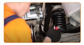
Release the coil spring by turning the lead screw of the coil spring compressor.
