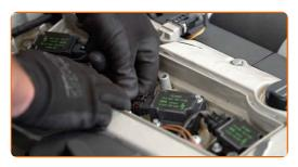
Unscrew the ignition coil bracket. Use a drive socket #E8.
