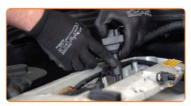
Tighten the ignition coil fastening. Use a drive socket #E8. Use a torque wrench. Tighten it to 9 Nm torque.
