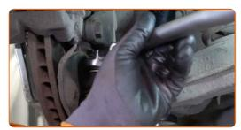
Tighten the fastener connecting the ball joint to the steering knuckle. Use a drive socket #21. Use a torque wrench. Tighten it to 105 Nm torque.
