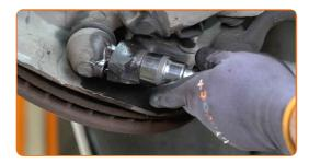
Disconnect the ball joint from the control arm. Use a ball joint puller.
