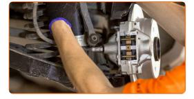
Clean the mounting seats of the stabiliser link. Use a wire brush. Use WD-40 spray.
