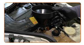
Pour coolant in the coolant reservoir.
