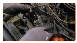
Remove the thermostat together with the housing.
