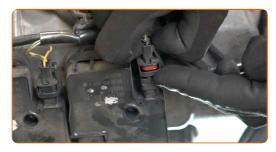
Remove the spark plug wire connectors from the spark plug wells. Use long round nose pliers.
