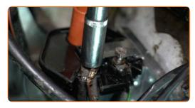
Connect the high tension cable to the ignition coil.
