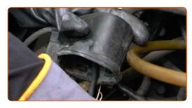
Disconnect the high tension cable from the ignition coil.
