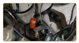
Screw in the ignition coil terminals. Use a drive socket #10. Use a ratchet wrench.
