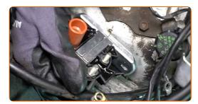
Screw in the ignition coil fasteners. Use a combination spanner #10.
