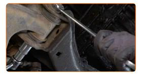
17 Unscrew the rear fastener of the control arm. Use a combination spanner #22. Use a drive socket #22. Use a ratchet wrench.
