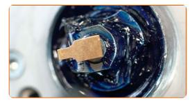
Install the hub bearing cap. Use a bush and bearing driver set.
