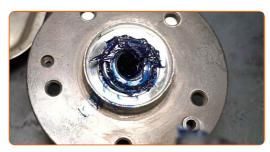
Reinstall the hub together with the new bearings.
