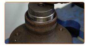
Treat the wheel bearings. Use bearing grease.
