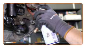
Unscrew the brake caliper bracket fasteners. Use a combination spanner #19.
