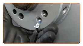
16 Remove the brake disc.
