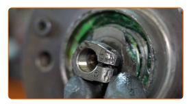
Remove the wheel hub together with the bearing.
