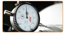
Adjust the axial clearance by tightening the adjusting nut. Use a combination spanner #22.
