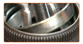
Clean the mounting seats of the wheel bearings. Use all-purpose cleaning spray.
