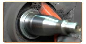
Remove elements of the bearings from the wheel hub. Use a bush and bearing driver set.
