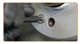
Tighten the brake disc fasteners. Use HEX No.H5. Use a torque wrench. Tighten it to 10 Nm torque.
