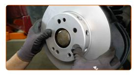
Remove the hub bearing cap. Use a crowbar. Use a hammer.
