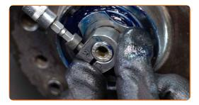
Treat the contacting surface. Use ceramic grease.
