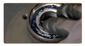
Install the wheel bearing oil seal. Use a bush and bearing driver set.
