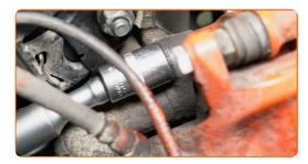
Clean the wheel rim mounting seat. Use a wire brush. Use all-purpose cleaning spray.
