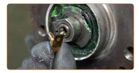
Loosen the wheel hub fastening nut screw. Use HEX No.H5. Use a ratchet wrench.
