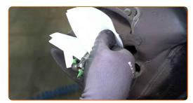
Clean the ABS sensor. Use a nylon cleaning brush. Use all-purpose cleaning spray.
