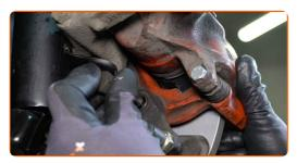
Tighten the brake caliper bracket fasteners. Use a drive socket #19. Use a torque wrench. Tighten it to 115 Nm torque.
