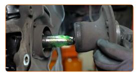
Clean the wheel stub axle. Use all-purpose cleaning spray.
