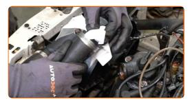
Unscrew the thermostat housing fasteners. Use a drive socket #10. Use a ratchet wrench.
