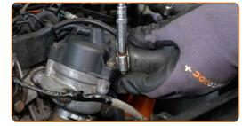
Connect the expansion tank hose to the thermostat housing.
