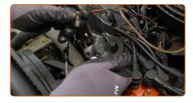
Remove the thermostat together with the housing.
