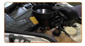
Pour coolant in the coolant reservoir.
