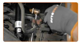
Unscrew the fasteners of the brake pad wear sensor wiring harness. Use Torx E10. Use a ratchet wrench.
