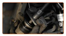
Attach the new wear sensor to the new pad.
