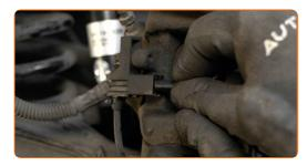
Install the brake caliper retaining spring.
