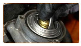
18 Install the thermostat housing.
