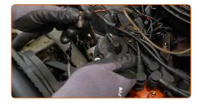
Remove the thermostat together with the housing.
