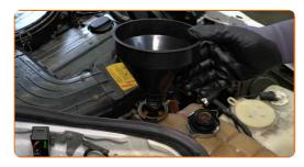
Pour coolant in the coolant reservoir.
