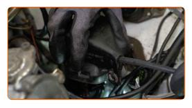
21 Install the high tension cable bracket.
