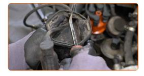
Insert the new high tension cable in the ignition coil cover.
