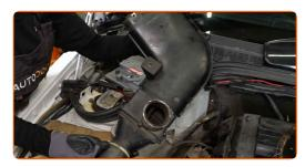
Remove the high tension cable bracket.
