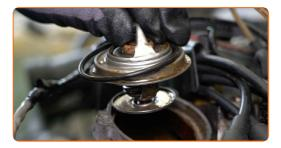
Replacement: engine thermostat – MERCEDES-BENZ S-Class Saloon (W126).
