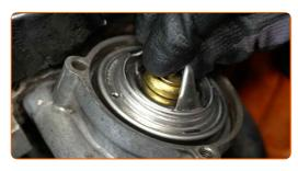
18 Install the thermostat housing.
