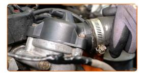
Secure the coolant hose clamp. Use a drive socket #8. Use a ratchet wrench.
