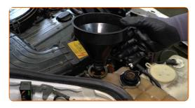
Pour coolant in the coolant reservoir.
