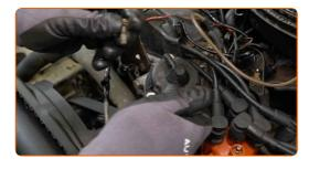
Remove the thermostat together with the housing.
