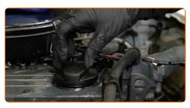
Tighten the oil filler cap.
