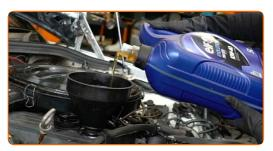
Replacement: engine oil and filter – MERCEDES-BENZ S-Class Saloon (W126).
