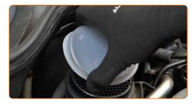
24 Install the air filter housing.
