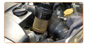
Replacement: engine oil and filter – MERCEDES-BENZ S-Class Coupe (C216) V6. AUTODOC recommends:
