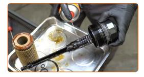
Install new O-rings and a new oil filter to their mounting seats on the filter cover.
