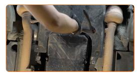
Put a waste oil container with at least 9 l capacity under the drainage hole.
