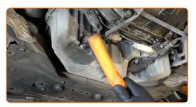
Unscrew the drain plug. Use a combination spanner #13. Use a drive socket #13. Use a ratchet wrench.
