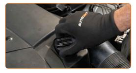
33 Tighten the oil filler cap.
